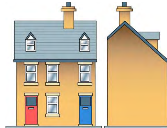
Figure 28: Placing of traditional dormers below the ridge line, away from party walls, in line with windows below and in neighbouring roof plane and set back from the eaves and gable.
