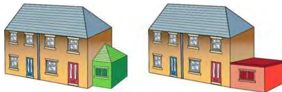
Figure 20: The left image shows a single storey extension proportionate and set back from the existing building line with an appropriate roofing design to match the existing house. The right image shows a poorly designed single storey side extension which is not set back from the building line and with a flat roof which does not match the existing house.
