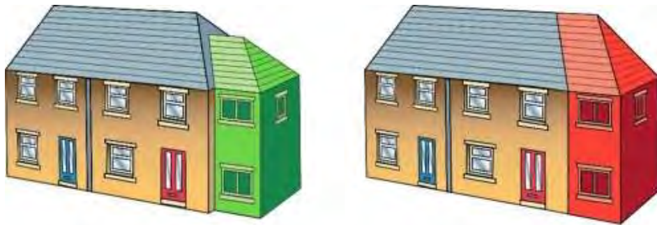
Figure 22: Left image shows a side extension which is set back from the existing building line and is proportionate to the existing building in scale. The right image shows a side extension which is not set back from the existing building line and is overly dominant in relation to the original building line.
